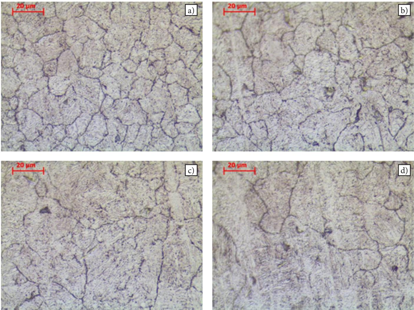
Fig. 4. Microstructure of steel 17-4PH after ageing at a temperature of 621°C: a) BM – fine-grained martensitic structure, b) martensitic structure, visible slight grain growth and c–d) weld – martensitic structure
