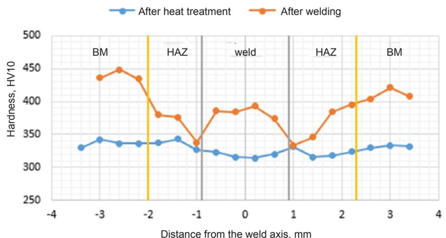
Fig. 6. Distribution of hardness (HV<sub>10</sub>) in the cross-section of the welded joint
