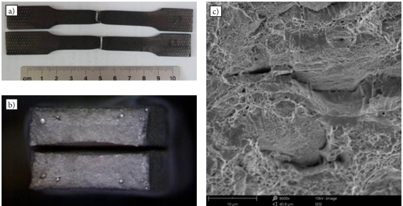
Fig. 5. Results of the tensile strength test of the joint made of steel 17-4 PH, after heat treatment (1038/621): a) specimens after rupture with the visible area of rupture in the weld; visible area reduction, b) specimen fracture (LM) and c) specimen fracture (SEM) – plastic fracture
