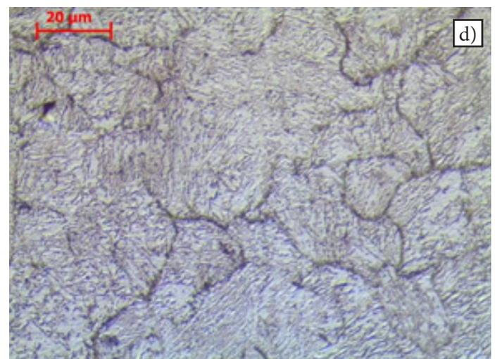
Fig. 3. Microstructure of steel 17-4PH after welding: a) BM – fine-grained martensitic structure, b) HAZ – martensitic structure with slight amounts of ferrite along the grain boundaries (indicated with the arrows), visible slight grain growth and c–d) weld – martensitic structure
