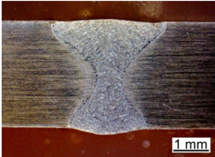
Fig. 2. Test joint macrostructure
