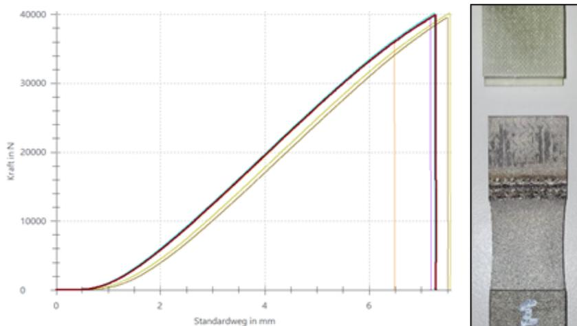
Fig. 8. Curve of displacement force in the tensile tests and the specimen after the rupture
