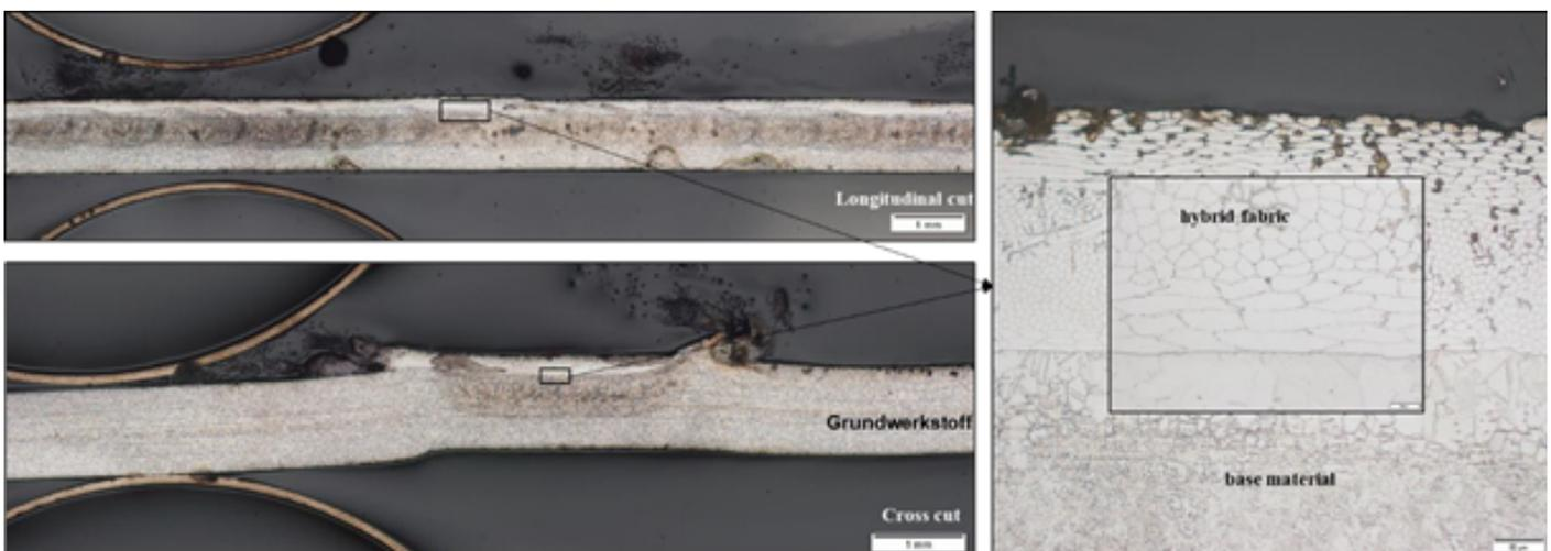
Fig. 7. Longitudinal section and the cross-section of the welded joint of the base material (metal) and the hybrid fabric
