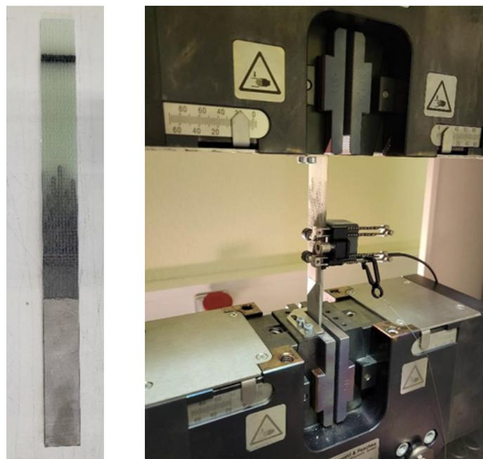
Fig. 6. Specimens having a length of 25 mm (a) and the tensile testing station (b)
