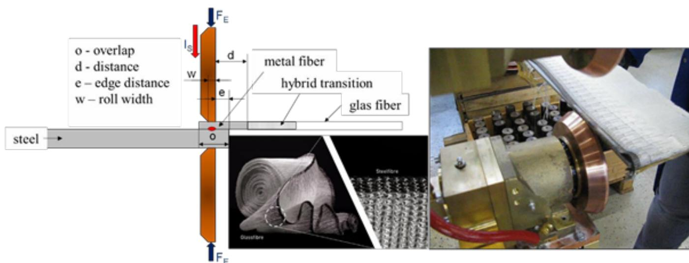
Fig. 4. Joining the metallic and the hybrid elements
