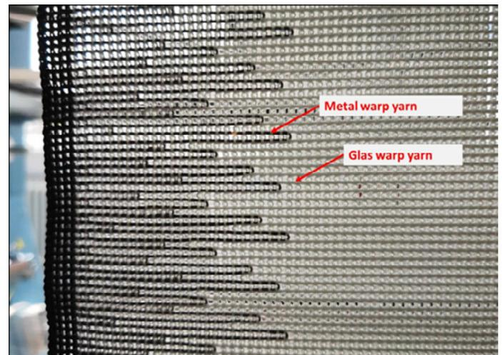
Fig. 2. Hybrid fabric composed of metal warp yarn (i.e. metal fibres) and glass war yarn (i.e. glass fibres)
