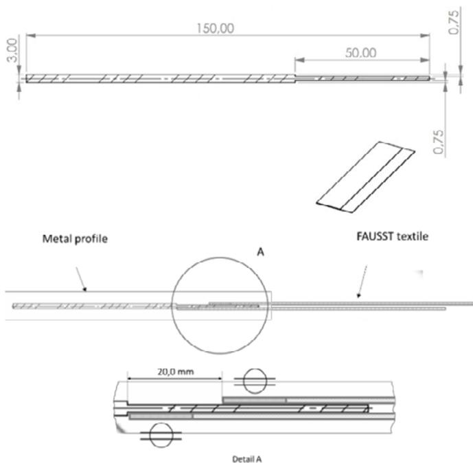
Fig. 3. Configuration of the element joining the FAUSST textile with the hybrid fabric on the metal profile and the milled metal profile for the element joining the FAUSST textile
