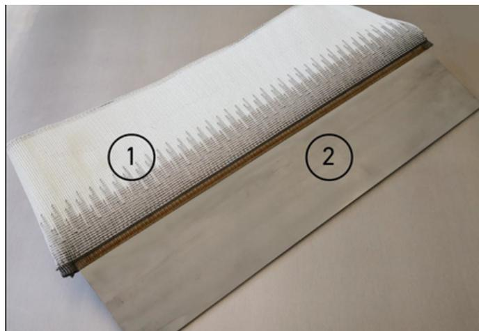
Fig. 1. Element made of the hybrid fabric and the metal profile: 1) one or more layers of the composite material and 2) metal profile
