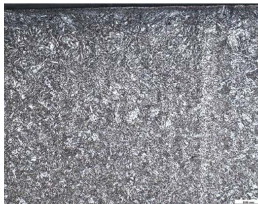
Fig. 3. Microstructure of the HAZ of the test element cut out of 20 mm thick S690QL steel using plasma; cutting in the air, a cutting rate of 0.50 m/min., mag. 200x [9]
