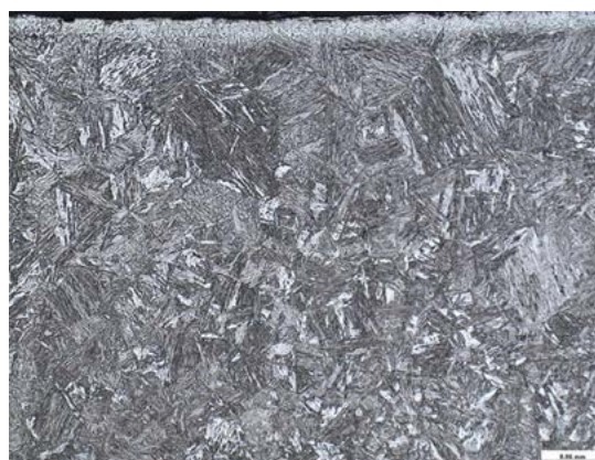
Fig. 2. Microstructure of the HAZ of the test element cut out of 20 mm thick S690QL steel using plasma; cutting in the air, a cutting rate of 0.50 m/min., mag. 200x [9]
