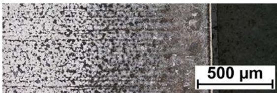
Fig. 9. Microstructure of the area after water jet cutting, v_c=0.16 m/min. Ferritic-pearlitic microstructure, etching with Nital reagent
