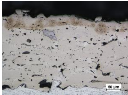
Fig. 10. Results of the microscopic tests of the coating made using the TungTec 10112 powder; magnification: a) 200x and b) 500x
