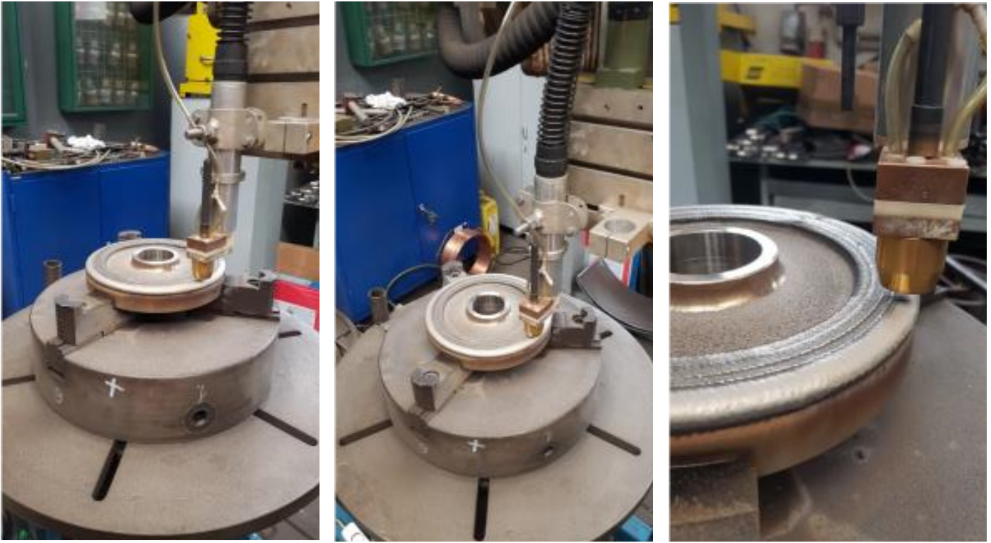
Fig. 21. Elements after the surfacing process performed using: a) DURMAT 61-PTA powder and b) and c) Höganäs 1559-40 powder
