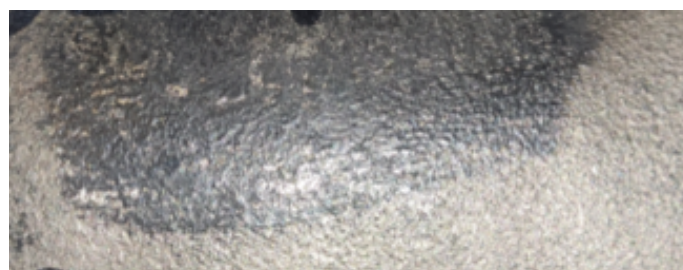
Fig. 15. Discolouration on the surface of the coating made using the Eutalloy RW 12112 powder
