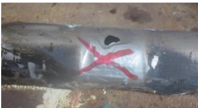
Fig. 1. Surface of 290 mm long cover plates after operation
