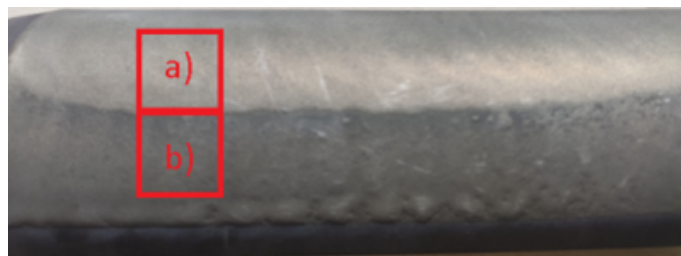
Fig. 2. Burnouts of the alloying components of the coating sprayed using the BoroTec 10009 powder; marked areas selected for chemical composition analysis (b – superheated area)
