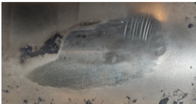
Fig. 13. Changes on the surface of the coating made using the Eutalloy RW 12496 powder
