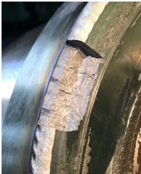
Fig. 22. Damage caused by improper machining
