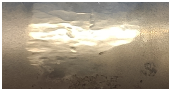
Fig. 14. Changes on the surface of the coating made using the Eutalloy RW 12496 powder
