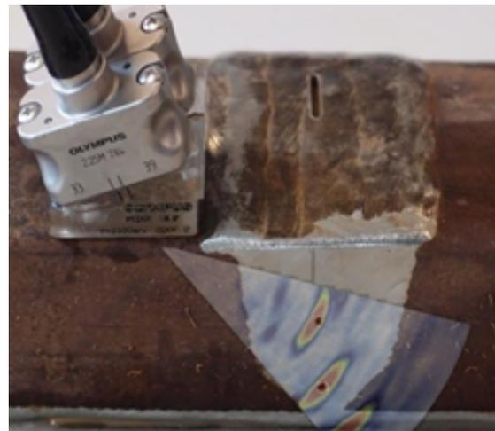
Fig. 6. Test performed using the PA technique and TRL transducers
