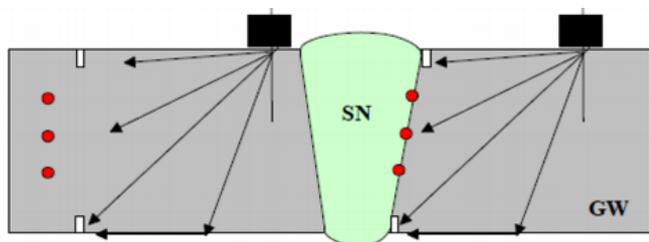
Fig. 4. Reference specimen with reference reflectors in the form of pass-through holes and notches (rectangular grooves)
