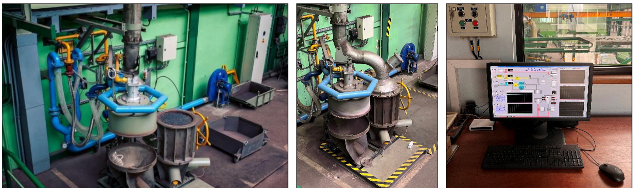
Fig. 5. Laboratory iron ore and waste sintering station with the process display system
